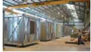
Factory producing volumetric units
